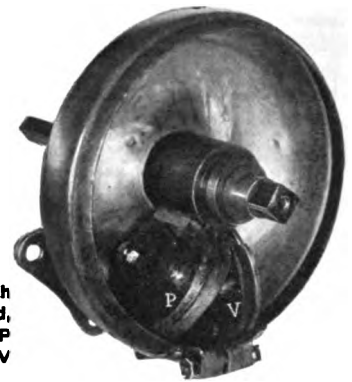
Stewart air motor with cover plate removed, showing rotating piston P and stationary vane V
